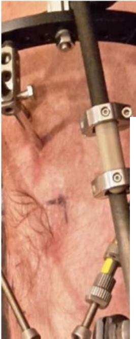
**Fig. 2.** Sensor prototypes attached to a strut of an external implant loading continuously and transmits data to the j
